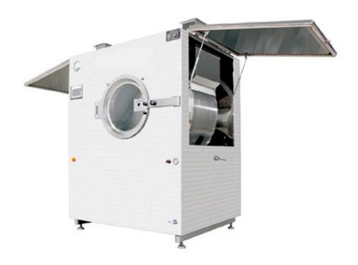
BG-80 high-efficiency coating machine is mainly used in pharmaceutical and food industries. It is a high-efficiency, energy saving, safe and clean equipment for coating tablets, pills and candies with organic film, water soluble film, slow and controlled release film and sugar film etc., which conforms to the requirement of GMP.
