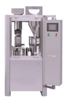
NJP-1200C automatic capsule filling machine is used for filling various capsules. Its output is 1200 capsules per minute. This pharmaceutical capsule filler can automatically complete positioning, separating, filling, waster capsule rejecting, locking and finished capsule ejecting. Automatic capsule filling machine is the ideal equipment for filling capsules especially in medium and small pharmaceutical factory, hospital preparation lab, and so on.
