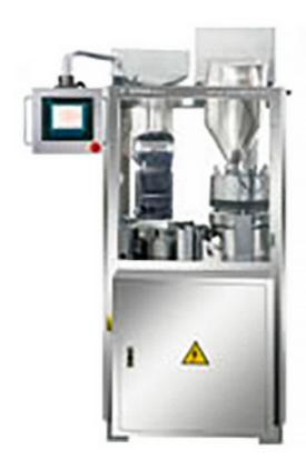
NJP-1200 fully automatic capsule filler machine, as a intermittent motion porous plug product, can automatically complete operations of sowing, separation, filling, waste capsule removal, locking, delivery and granule filling. With feature of reliable positioning, filling accuracy and high yield, this product is suitable for filling of powder and pellet shaped drug of small pharmaceutical companies. This product passes provincial technical appraisal and meets GMP standards.
