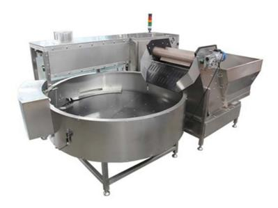
YLP bottle unscrambler is composed of carrying bottle part, bottle arrangement turntable, main bottle arrangement part, electronic control unit and pneumatic device.
