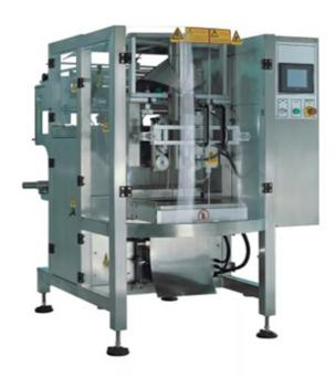
The Dustial Machinery® high speed vertical packaging machine made in China is an intermittent operating & high-speed vertical form fill seal machine. It's maximum speed is up to 100 bags per minute.
