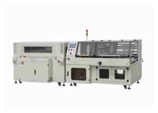
This equipment adopts side seal design, the side seal knife can seal continuously, the length of the packaged products is not limited. The height of side seal and cross seal can be adjusted up and down, and the sealing line can be adjusted to the center according to the height of the package, which makes the product packaging more beautiful. Wide packaging range, suitable for daily chemical, pharmaceutical, color cosmetics, food and other industries.
