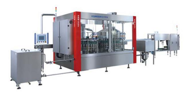
YSYGF series machine is capable of working under full-automatic conditions. The machines are applicable to the packaging production of milk, yogurt, milk beverage, fruit juice and so on, the completed full-automatically process is from vacuum negative pressure filling, cap-forming, capping, high-frequency sealing to product outputting.
