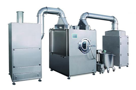
The machine is widely used for coating various tablets, pills, and sweets with organic film, water-soluble film and sugar film, etc. In such fields as pharmaceutical, food, and biological products, etc. And it has such characteristics as good appearance in design, high efficiency, low energy consumption, and small floor area, etc.
