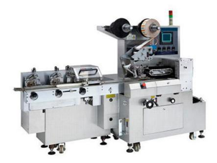
Horizontal pillow pack wrapping machine is an ideal packaging machine for soft, irregular, sticky or difficult handling product packaging and for multi packs as well.
