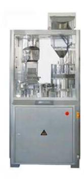
Z series Automatic Capsule Filling Machine is specially designed for drug filling of hard capsules, and various models of machines are available. It is widely used for filling different kinds of drugs due to its multi-purpose, perfect function, reliable performance and accurate filling. It has unique design and can complete the mixed filling of different drugs in the same capsule.
