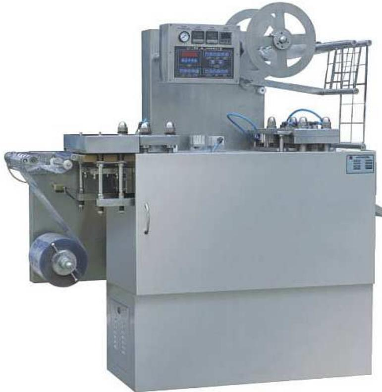
The auto plastic blown and forming die-cutting machine ZPQ-250 is a newly developed machine with success to meet the needs in the market by our own research fellows. It is characterized by ease of operation, lower energy consumption. It is suitable for forming foodstuff, medical equipments and the trays for electronic elements. It is integrated multi-functions like conveyor, blister forming, plate punch and counting displaying.
