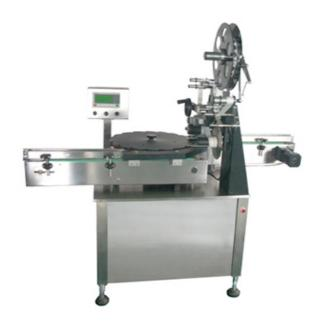
TTL-250 is suitable for labeling label on the caps of cylinder bottle.
