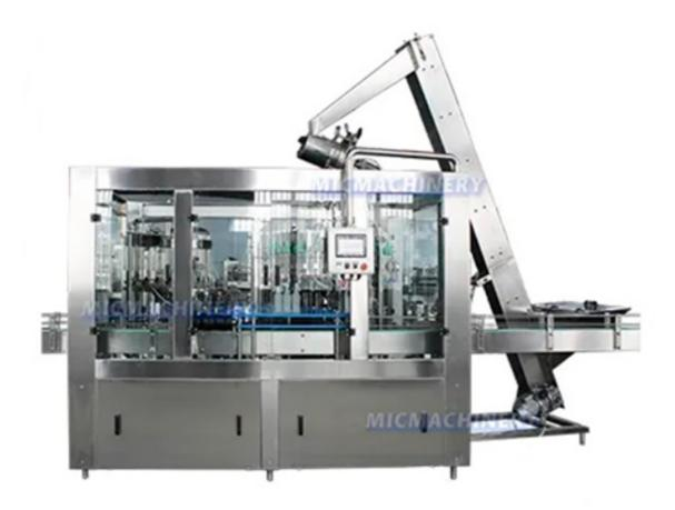
MIC-24-24-6 beer bottling equipment is applicable for equal pressure filler and capper of beer industry.
