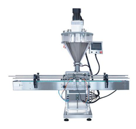
This machine is suitable for packaging fluidity Powdery product like milk powder, albumen powder, solid drink, white sugar, dextrose, coffee powder, rice powder, fodder, pharmaceuticals, agriculture pesticide, granular additive, dyestuff etc in bag, can, bottle package. Stainless steel design, in line with GMP standard, It can do measuring and filling work.
