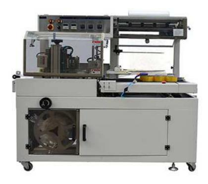
Automatic large-side sealing and cutting machine can be used for automatic online shrinkage packaging of products, automatic detection of products by photoelectric, automatic feeding or manual feeding mode can be selected, folding film can be used and sealing of other three sides. Thermostatic heating sealing and cutting system can be used for sealing and cutting PE, POF and other industrial standart.
