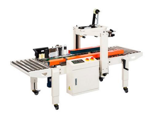
DFXC4030Cl carton sealing and labeling machine adopts adhesive tape and labelled paper to seal and label the carton. It can complete left and right carton sealing and side labeling at one time. Widely used in e-commerce, logistics and other industries, express packaging and delivery, sealing firmly, stick standard, fast speed. The machine is with counter, improves work efficiency.
