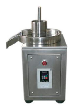
The machine is small desktop type hydro rotary granulator; it can produce granule of various specs from powdery materials.
