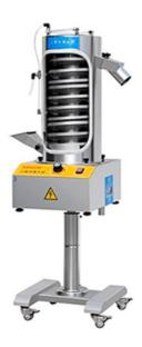
Model SZS230 Uphill Deduster also employed many new designs, to allow and to ensure a better and safer production, This Uphill Deduster is able to act as both elevating and dedusting machine, which made it a usual combination with other tablet-compressing machine and metal detection machine, and also made it extremely applicable in the field of pharmacy, chemical engineering, electronics, and food.
