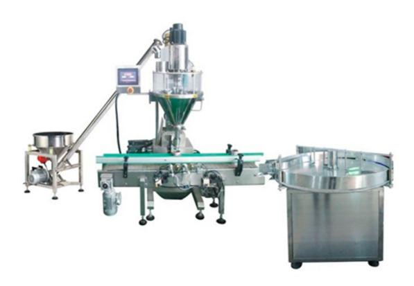
This machine is suitable for packaging fluidity Powdery product like milk powder, albumen powder, solid drink, white sugar, dextrose, coffee powder, rice powder, fodder, pharmaceuticals, agriculture pesticide, granular additive, dyestuff etc in bag, can, bottle package. Stainless steel design, in line with GMP standard, It can do measuring and filling work.
