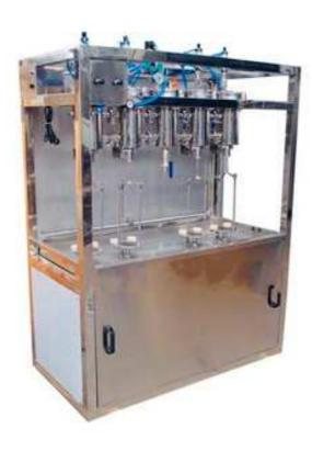
There is a certain pressure in the cylinder when the gas-containing beverage is filled, generally 0.2-0.4MPa. Here you can choose according to the type of beverage and the customer's requirements.
