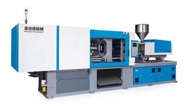
Master Packing joint with Ningbo injection company to supply customers with 10T-4,000T, injection weight 45g---40,000g, more than 30 kinds of specification injection mold machine. Master injection machine has energy-saving, environment-friendly, low noise, high rigidity, excellent performance, fast response, and high efficiency. With advanced servo motor and famous brand parts, Master injection machine becomes many customers' optimal choice for Injection needs.
