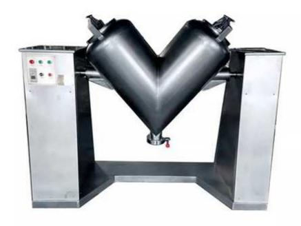
This machine is suitable for pharmacy and other industries, used for mixing the dry granule materials.
