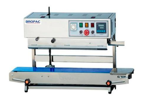
FRD series multi-functional film sealer (with solid inker printer) can be print the desired date date simult-aneously with sealing.
