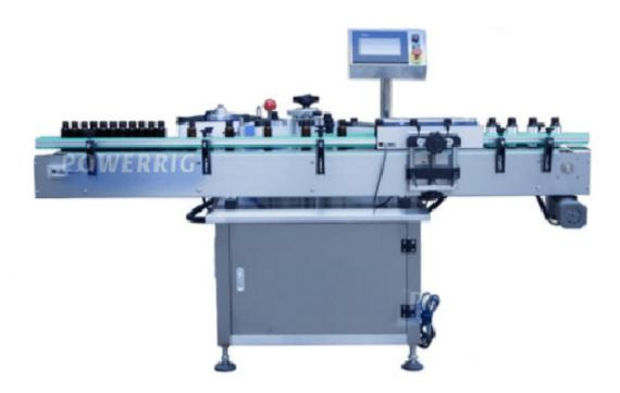
The machine in order to achieve reasonable production. Automatic labeling is very simple and fast. It can be labeled neatly and aesthetically. It can be used to label circular containers, such as pharmaceutical, chemical and food industries.
