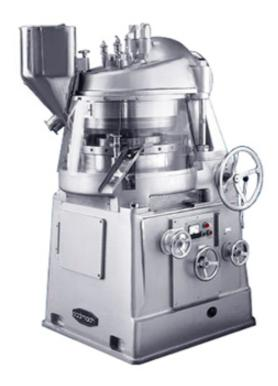
CRPP Tablet Press also known as RSII Press is a special designed heavy duty BOLUS press for producing very bigger sized tablets. It finds a vast application in industries like majorly Veterinary & Detergent, Ceramics, Powder metal, Chemicals etc. It is capable of making tablets uptil 63.5 mm diameter & 38 mm thickness. This machine has a 15 ton of compaction Pressure capacity. CRPP is offered in 14, 19 & 21 Stations Turret Configurations.
