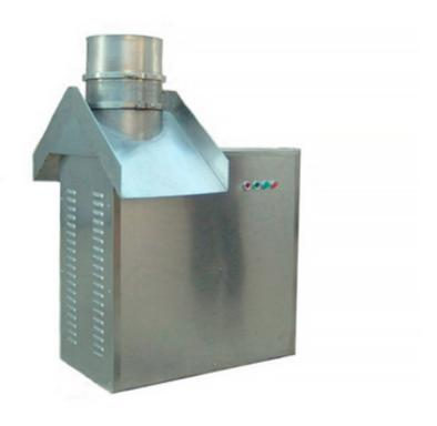
The machine can make necessary granule from the stirred raw material, it also can crush abolished slice and dry piece crowd it into granule. Especially, it is very suitable for raw material of higher viscidity.
