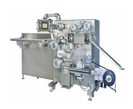
KW-B2 blister packing m/c applies the latest technology contribute to a low cost, low packing material consumption, low running cost, however the efficiency is extremly high. Precisely product loading apparatus creates a non-stop operational performance which in need of only one operator. KW-B2 suit for tablets, sugar coating / film coating, hard / soft gelatine capsule for blister packing.
