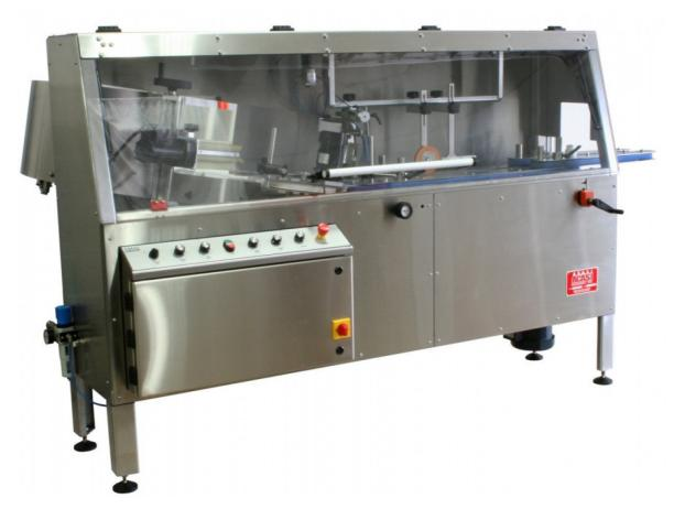
Automatic Bottle Unscrambler – Model TruSort-48 is capable of feeding and orienting plastic and metal containers.
