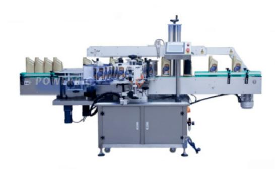
It is a single-side labeling machine, can be used for single-side and double-side labeling of flat bottles, round bottles, square bottles, such as single-side labeling flat shampoo bottles, lubricating oil flat bottles, hand sanitizer round bottles, can be installed on the labeling head, both sides are stuck together, improve efficiency, can be used in chemical, cosmetics, petrochemical, pharmaceutical and other industries.
