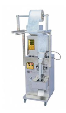
Powder packaging machine is suitable for quantitative, weighing, sub packaging, filling and packaging of tea, coffee powder, seasoning powder, pepper powder, chili powder and other materials.
