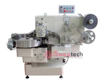
TBN820 Single Twist or Double Twist Candy Packing Machine with feeding disk for candies wrapped in double twist with one-two papers. The computer photo electric automatic detect, 100 percent of packing, no empty packs, Speed adjusting of frequency conversion.
