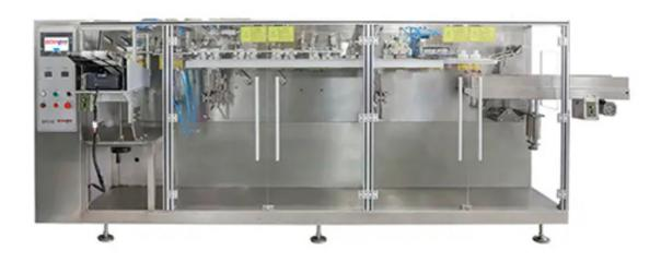
BHP-210 is specially designed for small and medium-sized bags. It can choose functions such as zippers or suction nozzles according to customer needs. The packaging capacity is 1200ml. The bag types are various in size. It is more convenient and fast to change the bag type. The packaging materials are diverse, including powder and liquid, solid, granules, tablets.
