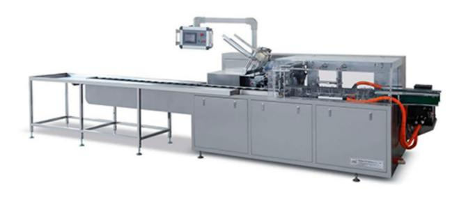
The entire packaging process of the horizontal cartoning machine is also divided into four stages: unboxing, opening, filling, and closing. Horizontal cartoning machines generally place the cartons upside down, and the products are pushed into the cartons from the side. This method requires the products to be relatively regular and easy to push. This type of packaging is used for packaging of facial masks, food, and daily necessities, and the products are output horizontally by a conveyor belt.
