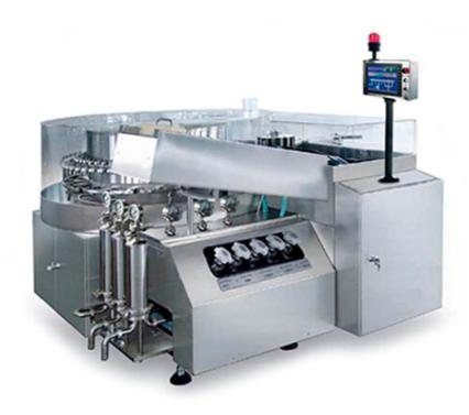
KCQ series vertical ultrasonic washing machine is the key machine type which our company is generalizing in recent years. The washing method is confirmed by our partners and users. It is widely used for washing of vials, ampoules, oral liquid bottles. Change part is easy to change.
