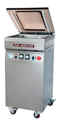
The vacuum chamber is all stainless steel for the utmost durability and cleanliness. DZ-400/2E is a mid-sized industrial-grade self-standing vacuum packaging machine. It's equipped with a heavy duty oil-filled rotary vacuum pump, a dual bar wide-seal sealing system, analog controls, and casters for ease of movement. Its chamber size allows it to be used of a wide variety of applications, as it can hold products of larger proportions.
