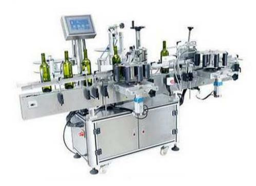
The adhesive sticker label machine is applicable for labeling various round bottles made of glass, plastics, metal and so on with accurate positions. Also a coder can be mounted on it to print such identifications as production date, shelf life and product batch number. The machine adopts an intelligent control system and an optimized design, thun featured by easy use and stable performance. In particular it's suitable for labeling and coding products with a small quantity but a great variety.
