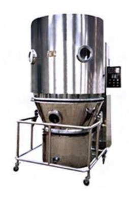
Purified and heated air is introduced from the bottom through suction fan and passed through the screen plate of raw material. In the work chamber, the state of fluidization is formed through stirring and negative pressure. The moisture is evaporated and removed rapidly and the raw material is dried quickly.
