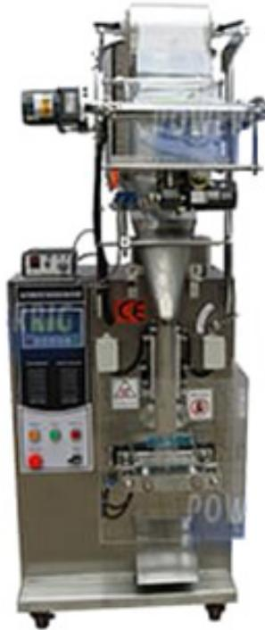
The sachet filling machine is a type of packaging machinery used to fill and seal small pouches or sachets with various types of products such as powders, granules, liquids, and pastes.
