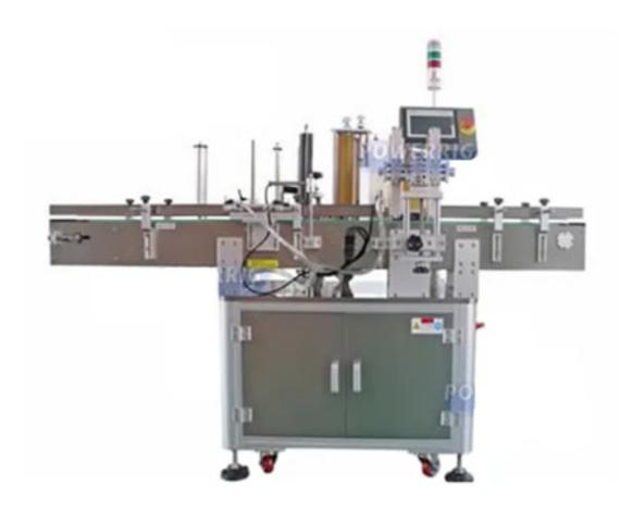
It can be used for labeling the whole cycle and half cycle of various round bottles, such as the labeling of round bottles of various specifications: round cans, round bottles, round cans, etc. in light industries such as cosmetics, food, medicine, daily chemicals, etc. The machine is composed of electric cabinet, conveying mechanism, bottle separation device, label rolling device, label brushing device, 1# label machine, operating system and control system.
