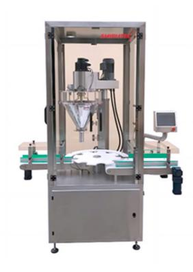
This series nutrition powder can filling machine could do work of measuring, holding, and bottle filling and etc, it can constitute the whole set bottle filling work line with other related machines.
