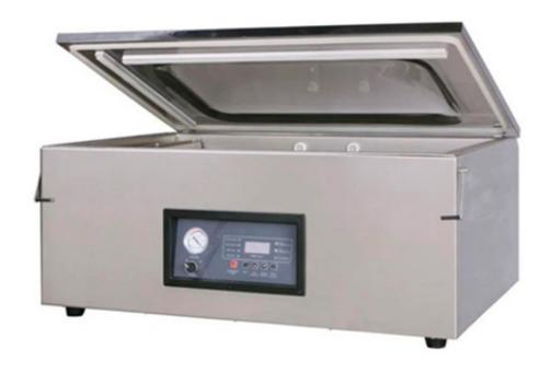
The DZ-900/T is a mid-sized industrial-grade counter top vacuum packaging machine. It's equipped with a heavy duty oil-filled rotary vacuum pump, a single bar wide-seal sealing system, and a modified atmosphere gas injection system. Its chamber size allows it to be used of a wide variety of applications, as it can hold products of larger proportions.
