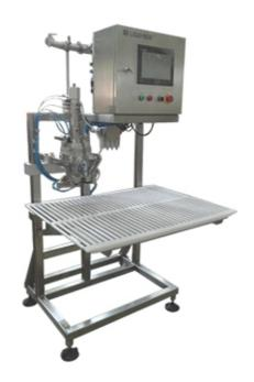
Bag in box aseptic filling machine is a high productivity, easy to use, compact filling equipment, suitable for all kinds of cover aseptic bags, such as ITW and Hoffer. It can used in food, medical, chemical and other industries to fill with milk, juice, carbonated drinks, chemicals and so on.
