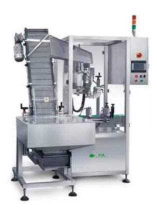
The machine is designed to position the bottles on the linear conveying line, and after pauses, the mechanical hand carries out cap feeding and cap turning of the positioned bottles. The machine can be used singly or for linked production. It is suitable for capping large bottles and barrels in such industries as medicine, food, chemical industry, daily chemical industry, etc.
