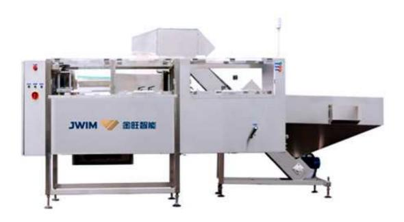
LP-200 Automatic bottle unscrambler machine has bottle elevator, unscrambling rotary plate, bottle-rejecting devices and unscrambling part, overturning bottle rejecting and electrical control cabinet. The machine is an improved model.
