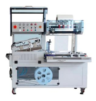
BSF-5640LG Auto L-Sealer is your best effective and economical choice for smart roomy facility layout. With packaging speed up to 25 PPM. Automatic L Bar Sealer is mainly applied to film wrapping for different products, which has the advantages of dustproof, damp-proof and beautiful sealing.
