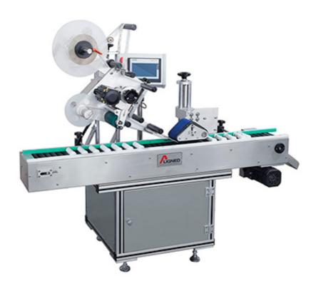
This equipment automatically completes the automatic feeding, positioning, labeling, pressing and ensures label consistent alignment, the action is accurate and stable. It is specially designed for high-speed bottling machines and can be operated online.
