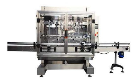
Automatic liquid filling machine is made with electric, mechanical and pneumatic principle. Use counter to control the filling column and designed with Special filling nozzle to reduce bubble when filling.
