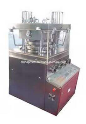
This machine is double-press type, continuous automatic tablet press for pressing granular raw materials into tablets. It is mainly used in pharmaceutical industry and also the chemical, food, electronic industries.
