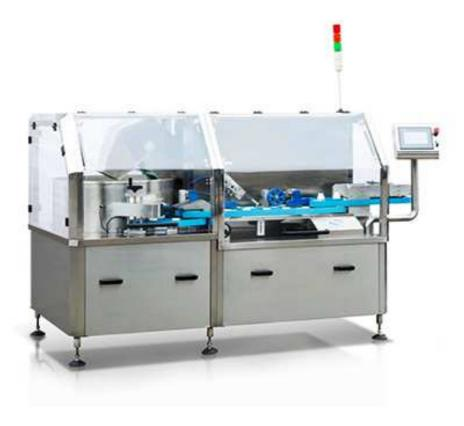
High speed unscramble is one part of the plastic filling line. Due to its high speed, it can be connected with other high speed production lines, also it can provide bottles for two bottle production lines at same time by two separate road transportation.
