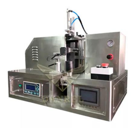
The process of tube sealing machine eliminates the use of glue and allows the thermoplastic parts to bond to itself. Ultrasonic sealing with the proper time setting and pressure is the fastest most reliable method for a variety of tube material sealing.
